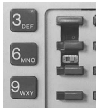
Dip to right: the 1 st station. Dip to left: the 2 nd station.
